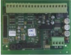
**STG-OUT16-S - Kidde Commercial - Aritech Fire - Modulo 16 out open collector ST.MTS**
